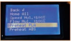
Warning: Extruder will now heat, do not touch the extruder while it is heated.
